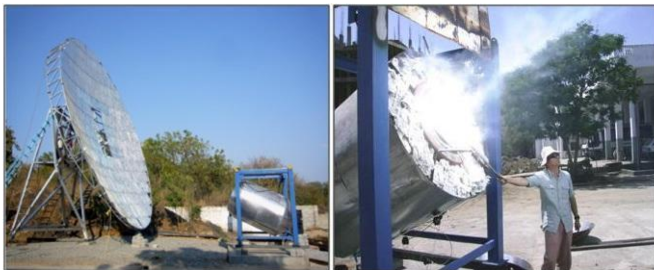
Figure 4: Prototype of the Scheffler Parabolic Dish with Cavity Receiver (left); first test of focus size and receiver (right).
