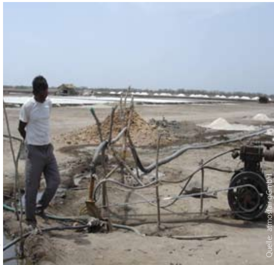
Water pump for salt mining with lower diesel consumption due to small technical modifications
