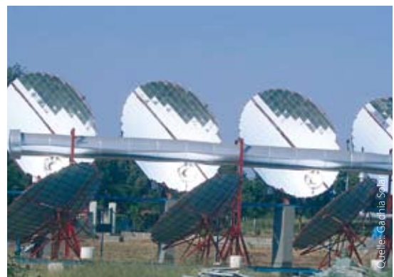
India: Solar mirrors to produce steam
