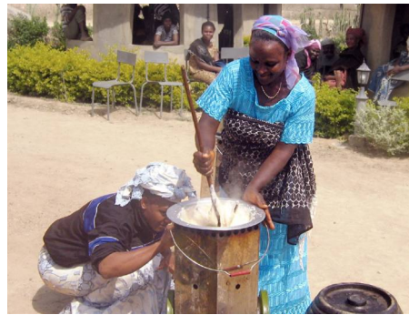
Efficient fuel wood stoves (Nigeria): The efficient stoves save about 80% of energy and help to reduce deforestation and indoor air pollution.
