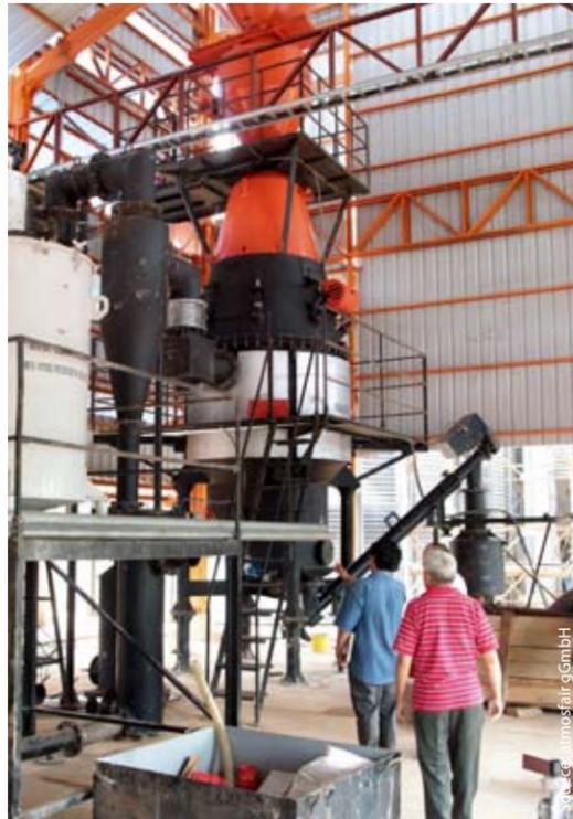
In the power station, Brazil nut shells are transformed into gas.
