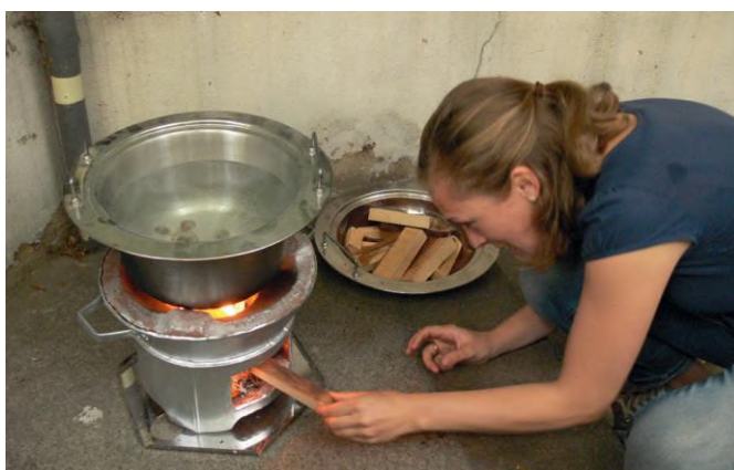
The atmosfair team testing the Dadin Kowa Stove
