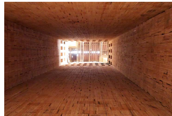
Rice husks are suitable as a more climate-friendly fuel for brick production. Below: View from below into the shaft of a VSBK.
