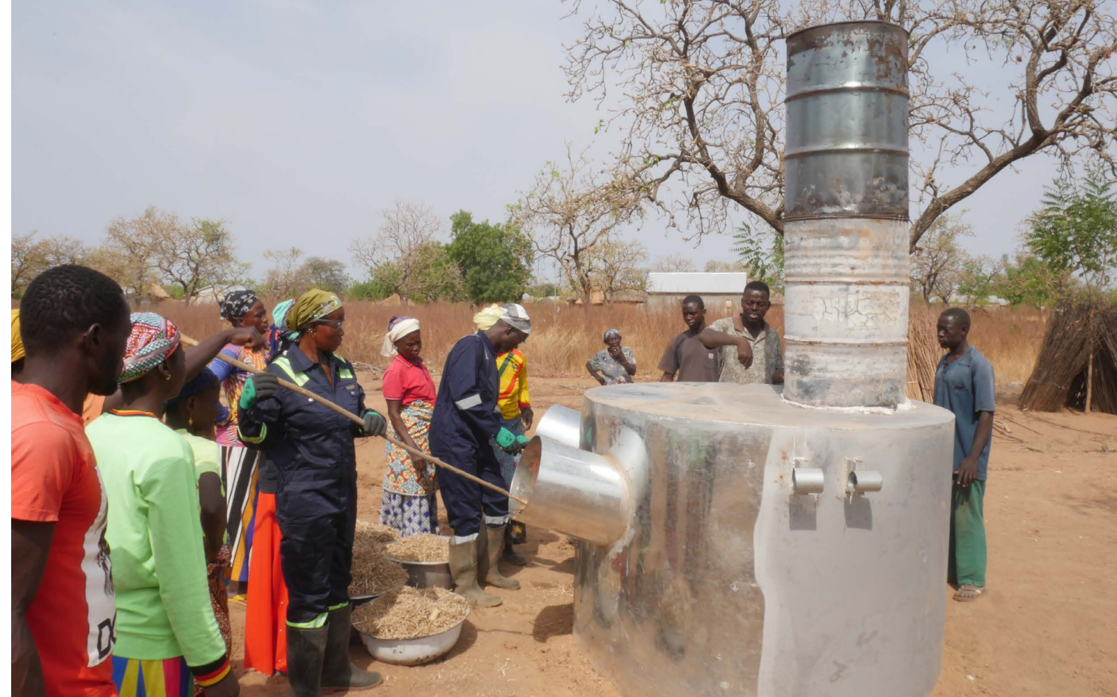
In Ghana, farmers turn crop residues into biochar. To do this, they use small pyrolysis units provided by atmosfair.
