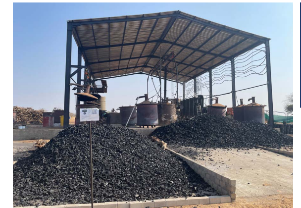
In this plant, atmosfair, in collaboration with PyroNam, converts shrub cuttings into biochar.
