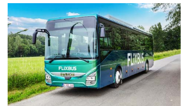
The Iveco gas-powered bus that is in service in the BeNeLux countries. The bus is operated exclusively with biomethane made from waste materials. ©IvecoBus
