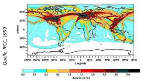
In March 2011 it was made 'official': The cirrostratus clouds and condensation trails created by aircraft contribute to global warming. This has been scientifically proved in detailed calculations used in a new study by the German Aerospace Center (DLR). According to this, the radiative forcing (rf) and thus the global warming effect of these artificial clouds is almost 40mW/m2 and is therefore more than that of the entire CO2 emitted by air traffic since the middle of the 20th century.
